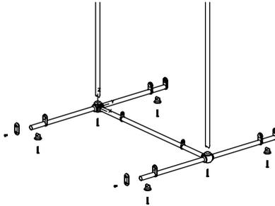
In this Photo Put 2 other pipe with its L & Key from down & then Fix the other casting pc's all the side & then put the Leg with its L & Key all 4 side & Fix all L&Key very Tight.
