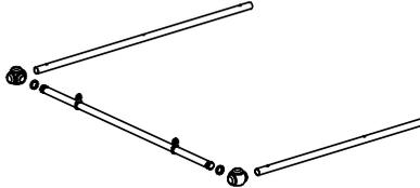
First Step you see the Photo there are 2 same pipe & one pipe is different then take 2 big Casting pc's with its Check Nut & Put this 3 pipe in its same like photo.
